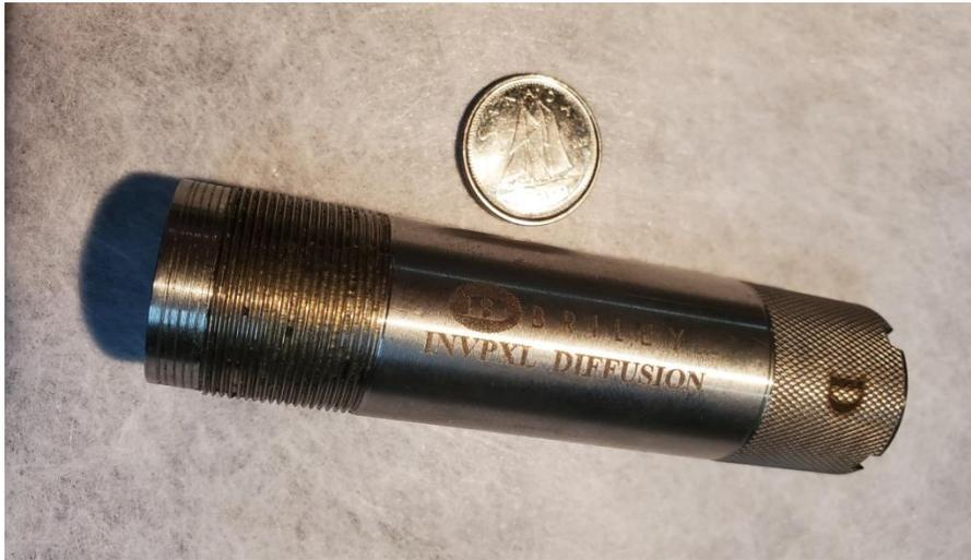
Often called a "Spreader" choke (S), sometimes referred to as a "Diffuser" choke (D) this is a choice for skeet's low targets that are coming towards you, sporting clays' rabbit and some springing teal targets. A negative choke has an inside diameter greater than the barrel's bore. To help achieve this greater diameter, negative chokes often extend beyond the muzzle. Patterns open fast and wide, making it easier to connect on "up close and personal" targets.
