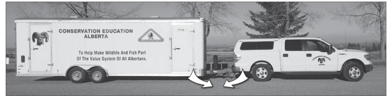
Without weight distribution. Note how the weight of the trailer is carried forward toward the front of the trailer and the rear of the truck.
