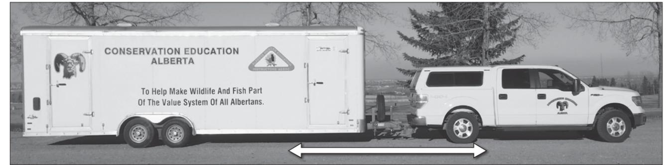
With weight distribution bars. Note how the weight of the trailer is more evenly distributed.
